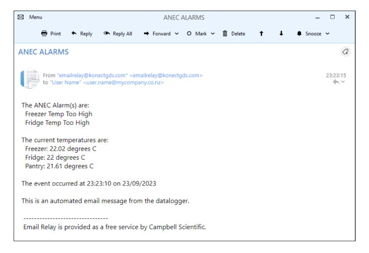
The datalogger can send alarm email messages advising users of events occurring at the station that need prompt attention. All messages are in the same format which is designed to alert users by the subject line alone, with more information contained in the message body. The format is designed to ensure messages are readily identified in a users email In-Box even on the smaller screens of mobile phones. A sample email message is shown above.
