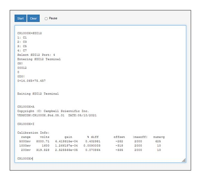
The terminal function is primarily an engineering tool. It is not necessary to use it for routine datalogger operations other than configuring SDI-12 sensors. A sample Terminal session is shown above.
