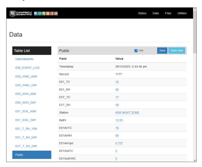
The Data page enables data tables stored in the datalogger to be viewed and downloaded. On some datalogger models this page also allows selected variables to be graphed in realtime. It can be selected by clicking on Data on the header/menu bar at the top of the page.
