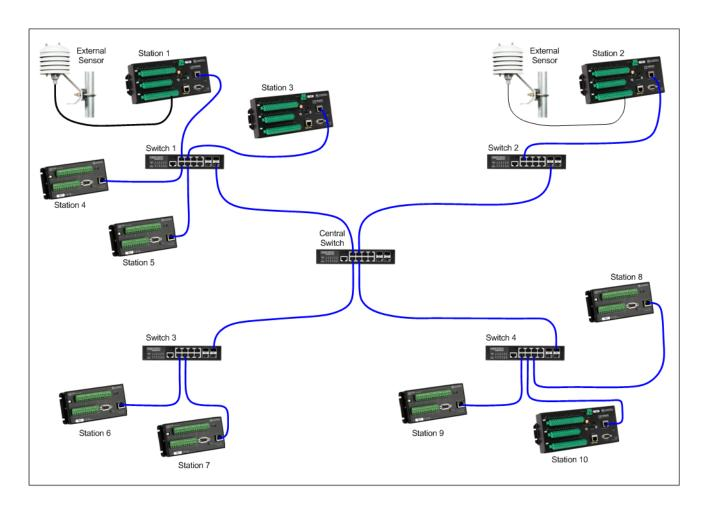
A good design technique is to keep communications between stations localised, as much as possible, to the network switches they are directly connected to.
