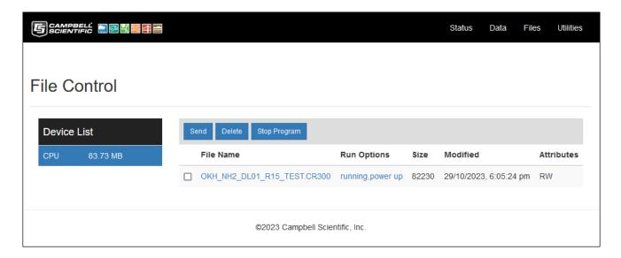
The File Control page enables management of the datalogger files. Files can be sent, deleted, activated, and deactivated. The files page can be selected by clicking on Files on the header/menu bar at the top of the page.
